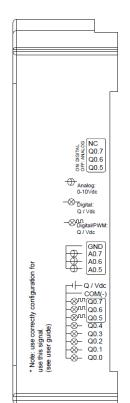
Configuration Switch\* (see section 8 to select the correct configuration for outputs).
