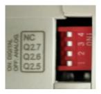
For the Analog Shield (Zone B & Zone C) if a switch is set to ON, it can only act as Digital Output. If it is set to OFF it can only act as an Analog Output.
